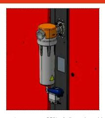
Moisture separator removes 65% of all condensable moisture via electronic Zero Loss condensate drain valve. Dry alarm contacts provide peace of mind.
