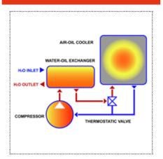
RVX45-75UPRareair-cooled compressors with an integrated Heat Recovery System for process water heating. Recovers up to 80% of mechanical energy (equivalent to more than 70% of electricity consumption required at mains) into hot water. Maximum outlet water temperature: 65-70°C/149-158°F.
